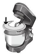
Place the SPLASH GUARD onto the top of the STAINLESS STEEL MIXING BOWL. Once all attachments are secure, push the TILT RELEASE LEAVER to the RIGHT to lower the MIXER HEAD.
