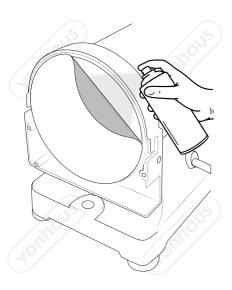
Remove the old Sanding Disc using a solvent remover.
